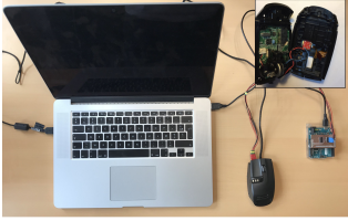
Figure 1: Our setup comprises a Logitech G9 Laser Mouse connected via USB to the host computer with the MPU-9250 chip embedded inside. The MPU-9250 chip is connected to an Arduino Leonardo that is connected to the host computer via USB.
